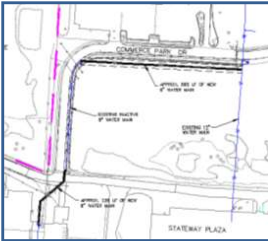
MAP SHOWING PROPOSED WATER MAIN EXTENSIONS ON COMMERCE PARK DRIVE
